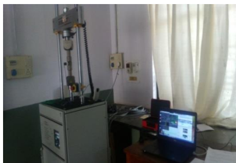
Figure1.8: Universal Testing Machine (Axial)
