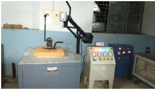
Figure 1.1: Resistance furnace used for stir casting
