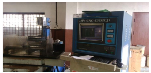
Figure 1.7: Wire EDM used for Notch Preparation
