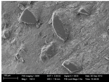
Figure 1. 3: Microimages of Al2219-3 wt%B 4 C-3 wt%MoS 2
