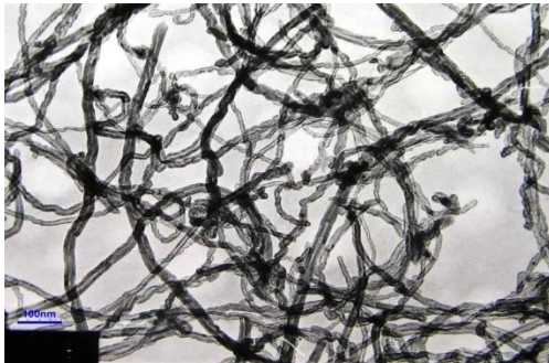
Figure 1.1. a) TEM of MWCNTs
