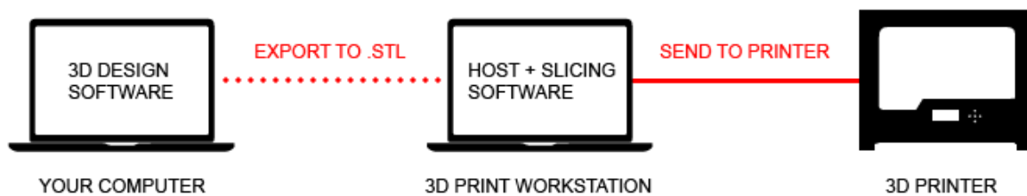
Figure 1.1: Process involved in 3D Printing
