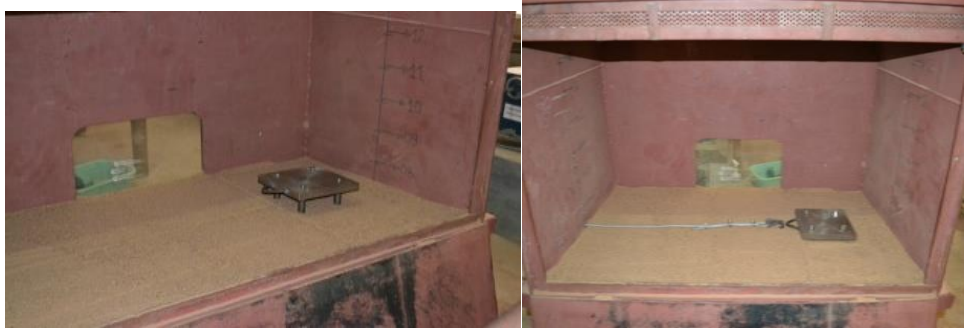
Fig.4 Model box with Pile Group Combinations
