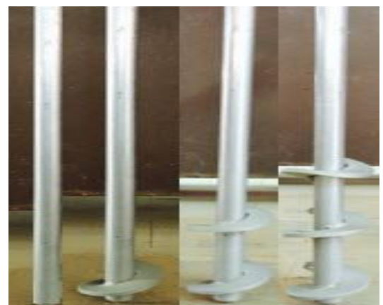
Fig. 2: Schematic diagram of experimental set up Fig. 3: Model Pile and Helical Piles
