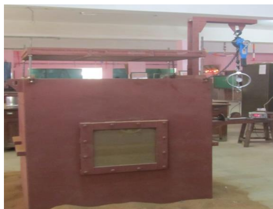
Fig. 1: Photograph of Model Test Tank, Lever Hoist, and Proving Ring and LVDT arrangement with Sand Pouring Box
