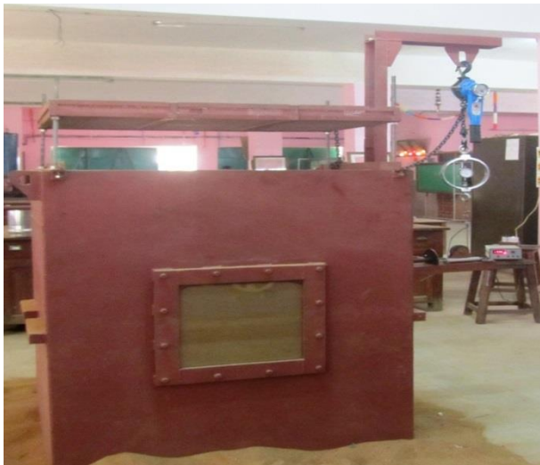
Figure 1: Photograph of Model Test Tank, Sand Pouring Box, Lever Hoist, Proving Ring and LVDT arrangement
