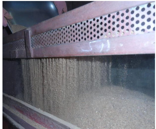
Figure 2: Rainfall Technique by Sand Pouring Box
