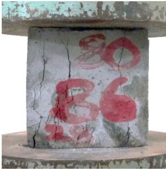
Fig-3: Cube Specimen Failure under Compressive Loads
