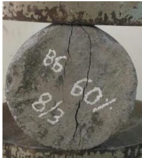
Fig-5: Cylinder Specimen Failure under Tensile Loads
