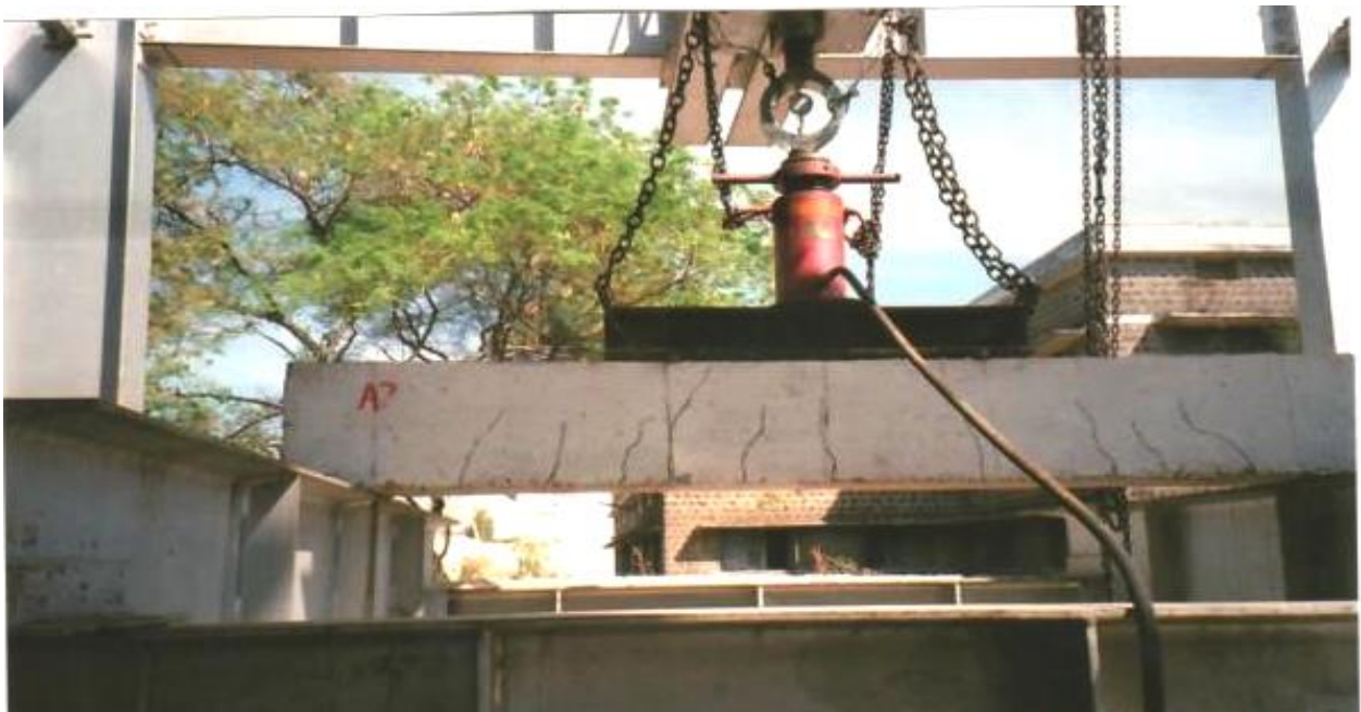
Fig.4. Testing of reinforced geopolymer concrete beams under two point loadings- B15
