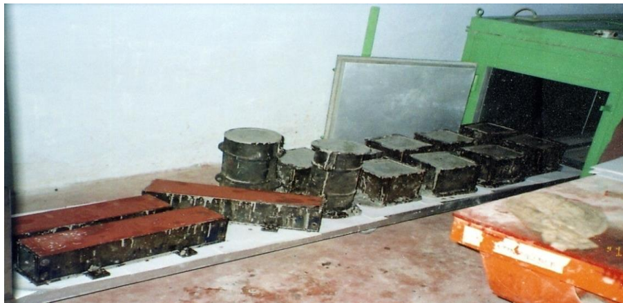
Fig.2. Oven dry curing of Cubes, Cylinders and Prisms
