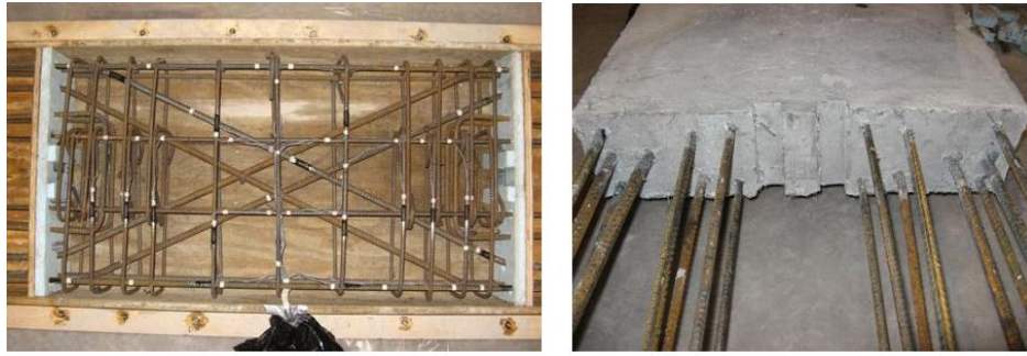
Fig 10. Precast Coupling Beam – Cold Joints [18]
