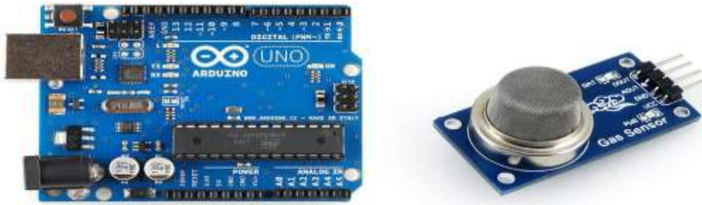
Figure1. Arduino UNO microcontroller and MQ-6 Sensor
