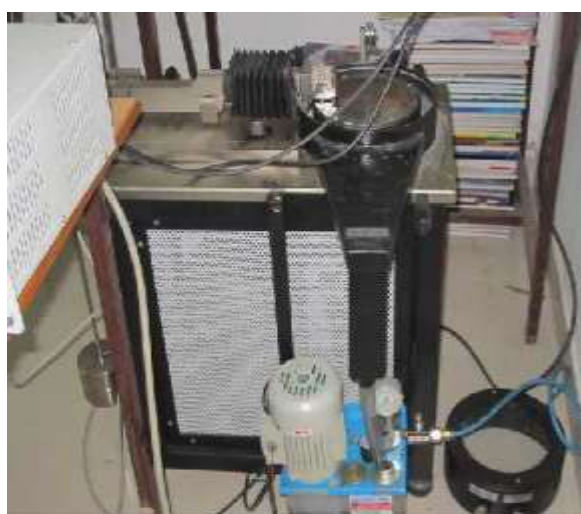
Fig 3.1: Photograph of pin on disc wear testing machine
