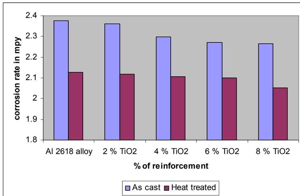
Figure3. Effect of heat treatment on corrosion rate.
