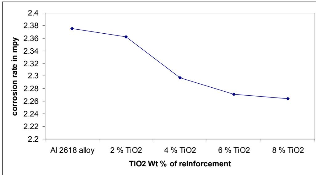
Figure 2. Effect of reinforcement on corrosion rate of composites.
