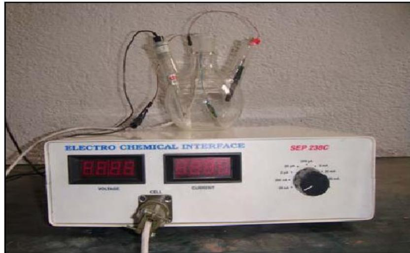
Figure 1. Electrochemical test rig SEP 238C model.
