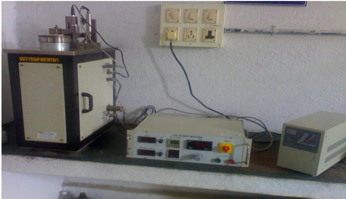
Figure 1. Dry sliding wear test rig.
