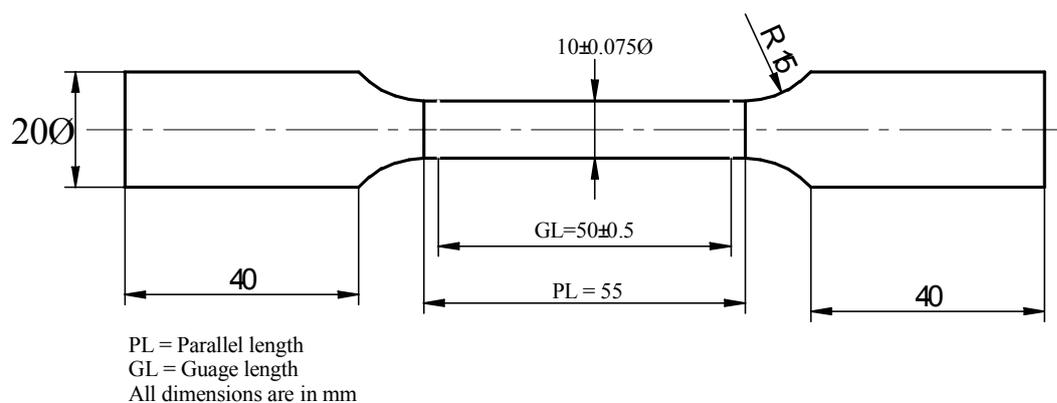
Figure 1 Tensile test specimen
