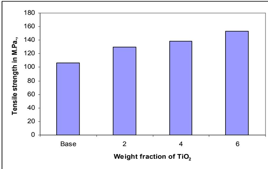
Figure 5 : Tensile strength of Base material and TiO<sub>2</sub> composite
