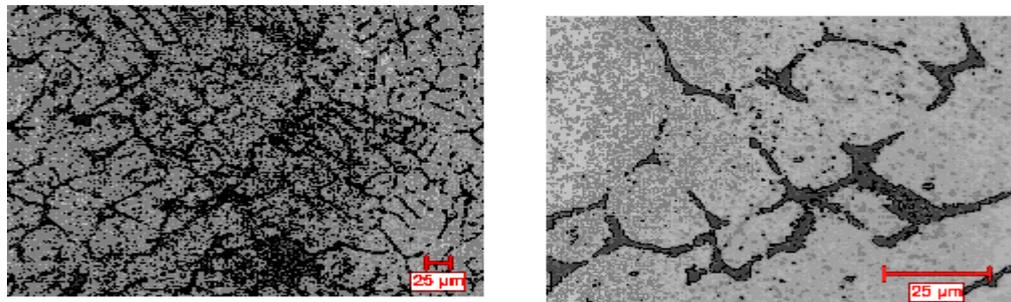
Figure 3 Optical microscopy cross – sectional view of T6 heat-treated Composite containing 6-weight % of TiO<sub>2</sub>
