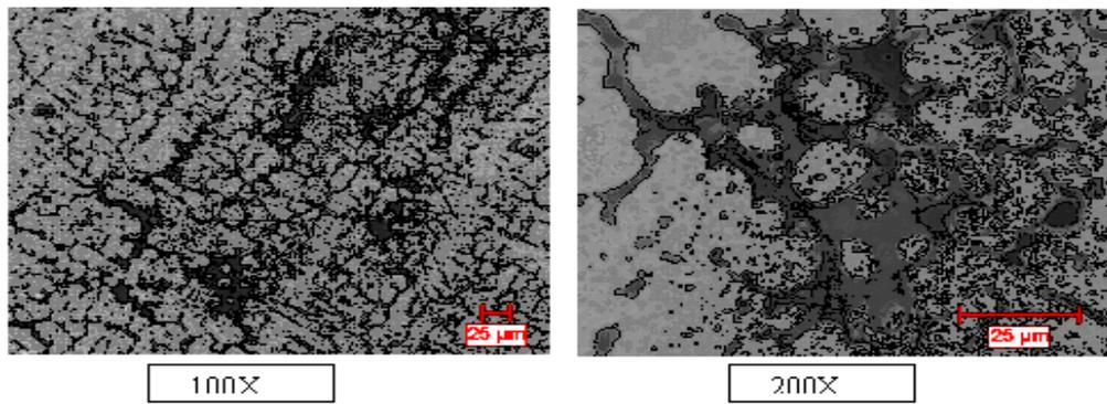
Figure 2 Optical microscopy cross – sectional view of Al 2618 alloy
