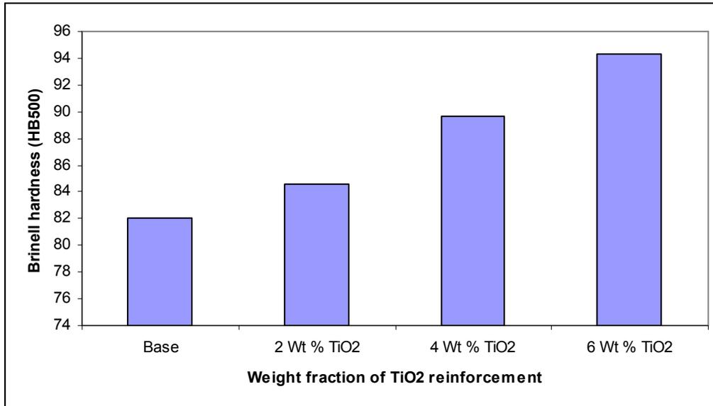
Figure 4 Hardness of Base materials and TiO<sub>2</sub> composite
