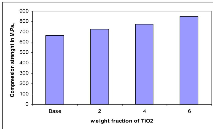
Figure 6: Compressive strength of Base material and TiO<sub>2</sub> composite
