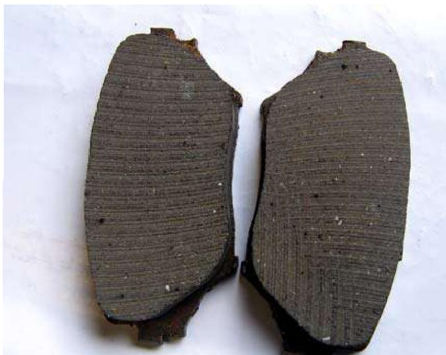
Photo 3.0 (c) Plate of perform and finished CNS-based friction composites.
